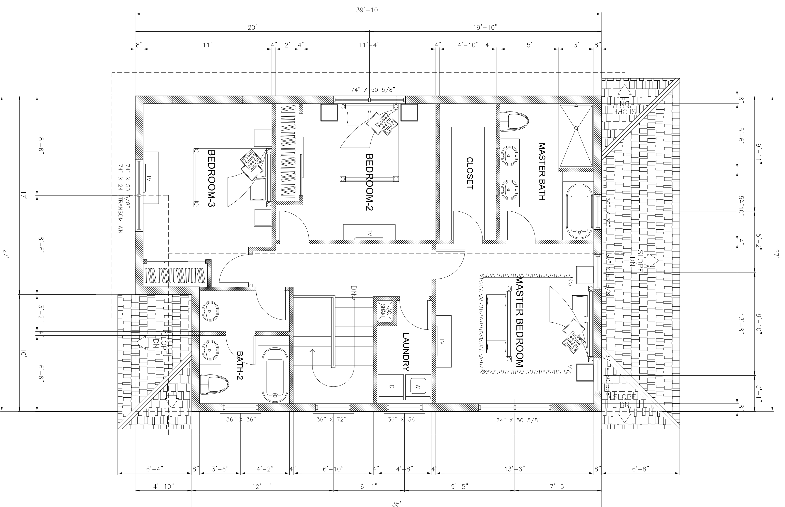
BUILDING #9 MODIFICATION 02 SECOND FLOOR PLAN 1,027.00 SQ. FT. A2.1 SCALE 1/4"=1'-0"
